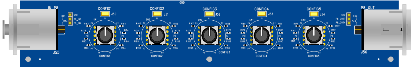
Figure 12: Dunglass Rotary Switches for Hardware Control Mode
